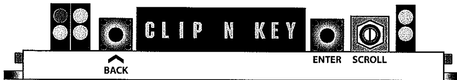
The front of the MegaKey card has a display, buttons, and a scroll knob that is used to get information about the device.
