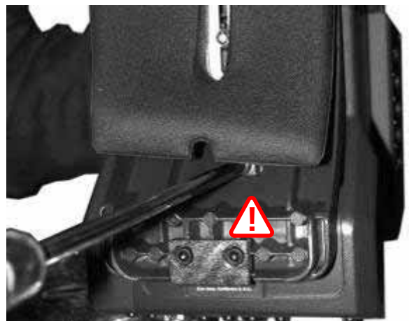
4. Tighten bottom camera screw under shoulder pad.
