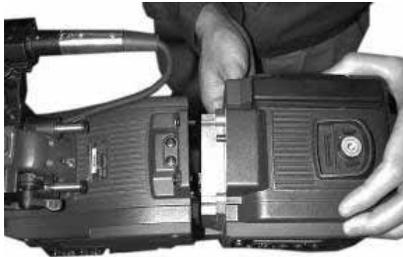
1. Align Z-DR1 with camera & support from bottom.
