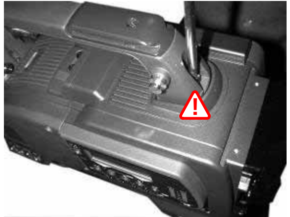
6. Tighten front and back screws of camera handle.
